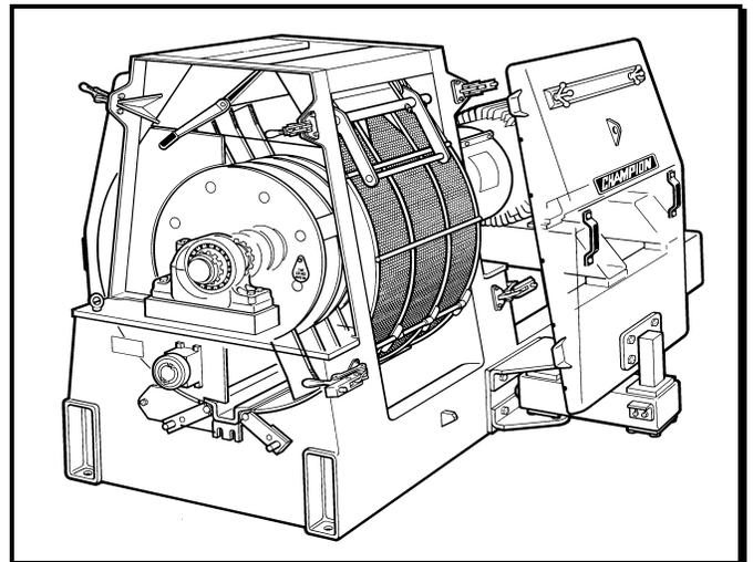
screen design will permit the user to adjust the screen sizing on the down side and up side to maximize productivity and product quality. A “Regrind Chamber” at the bottom of the mill introduces enough turbulence to swirl materials back into the hammer path at the 6:00 position. This regrind chamber must be large enough to take product out of rotation as the hammermill operates, but should not be so large as to reduce the available screen area significantly.
