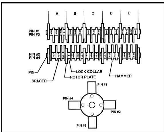
Hammer patterns (the number and distribution of the hammers on the rotor) and positions (setting the hammer closer to or further from the screen) have a profound effect on the performance of any hammermill. Because different materials grind differently, the ideal number of hammers and clearance to the screen will need to be adjusted according to each application.
